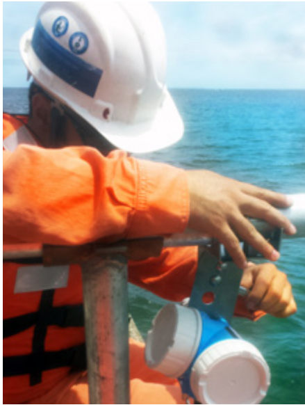
A HidroMares technician prepares a YSI Nile 502 radar water level sensor, part of the company's innovative SISMO® harbor monitoring system.
